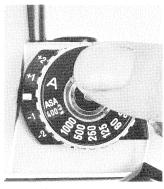
Need auto-exposure compensation? Just match the A on shutter speed dial to the correction needed. Here it's set to +1 EV.
