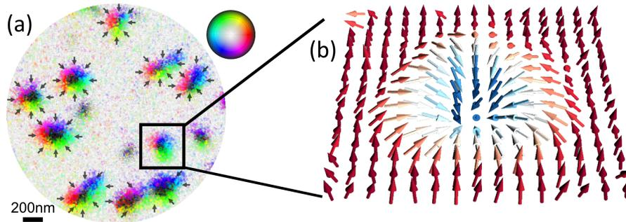
**Figure 1** (a) SPLEEM image of skyrmions in magnetic multilayer designed to stabilize ambient-temperature skyrmion phase [5]. Magnetization vector orientation rendered in color according to color-wheel. (b) Single skyrmion image, 3D vector array shows magnetization at image pixels.
